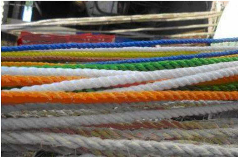
Figure 3. Ropes made from waste polythene papers and sisal.
